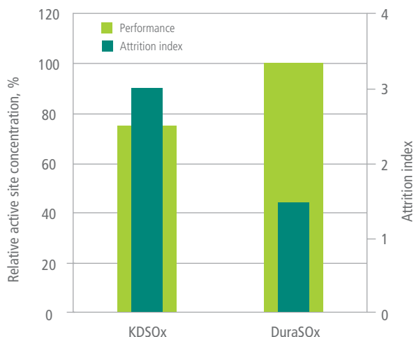
Figure 2: Attrition resistance improvements provide the opportunity to add more active ingredients and boost performance.
